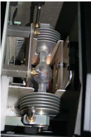
Modern followspot with double side HMI Bulb (4KW HMI from Robert Juliat)
